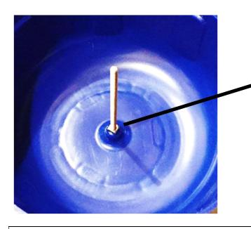
Tighten the last square nut bottom of the bowl. This will keep the tumbling bowl its place. Check the tightening by hand every time before start tumbling
