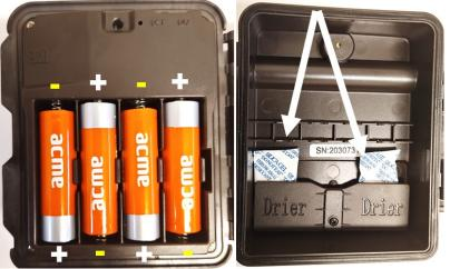
Insert good quality AA alkaline batteries (4pcs 1.5V AA), note polarisation (+/-)
