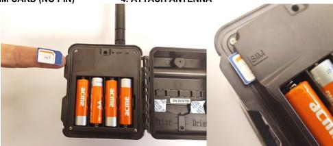
SMS Trap Alarm supports mini SIM card size. Take OFF PIN code request from SIM card before inserting it to unit.
