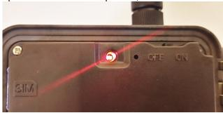
The red LED light is ON for about 3 minutes, after which it turns off and the device is activated
